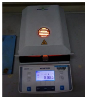
Fig. 11. Mettler Toledo Moisture Analyzer in Process
