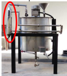
Fig. 3. Location of Condensing Chamber
