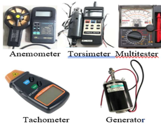
Figure 2. The measuring instruments used for testing
