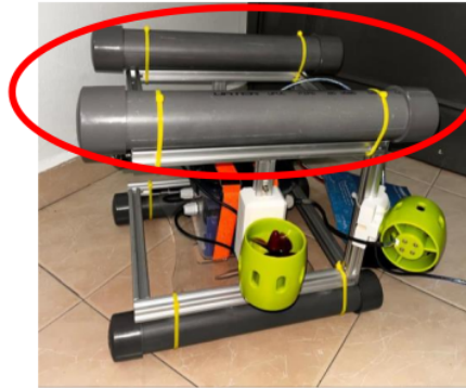
Fig. 3. Upper PVC Pipe (Buoyancy Tank)
