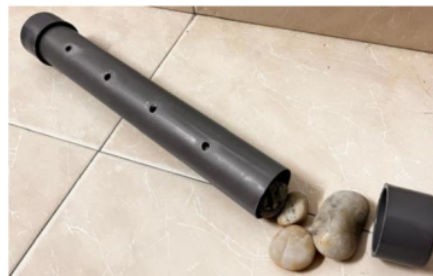
Fig. 4. Bottom PVC Pipe (Ballast Tank)
